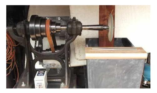
I have setup this lathe with variable speed in addition to the pulley speed changes. This allows for full torque at all speeds. In addition, I have welded up the steel base to hold up to five  $8^{\circ} \times 8^{\circ} \times 16^{\circ}$  concrete blocks to add mass to the unit. The tub is an old lab sink mounted on a table separate from the lathe.
