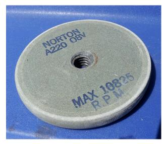
Notice that on the backside of this wheel, the lead has been carved down to the surface of the wheel to allow this wheel to snug up against the stabilizing flange of the lathe spindle or extension.
