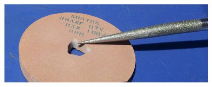
This process may also be done with a tapered round diamond coated file – dry. If the arbor hole is too small for my needs, I redrill it to the desired diameter using a diamond coated core drill on an old drill press. This process is done wet. This roughing up of the arbor hole is necessary for the lead to firmly grip the walls of the arbor hole. It is this firm grip of the
