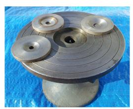
The device shown is by Spatzier and the cast iron base allows for leading a variety of wheel sizes. There are three included inserts which form the lead shoulder when casting the lead. The insert may be removed and the molten lead cast with the depression
