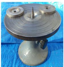
The larger the arbor hole in the wheel, the larger holed insert to be used. In these pictures it can be seen how smaller wheels use only the tip of the threaded spindle. As the wheel gets larger, the thicker portion of the spindle is used (to add additional support to the wheel.
