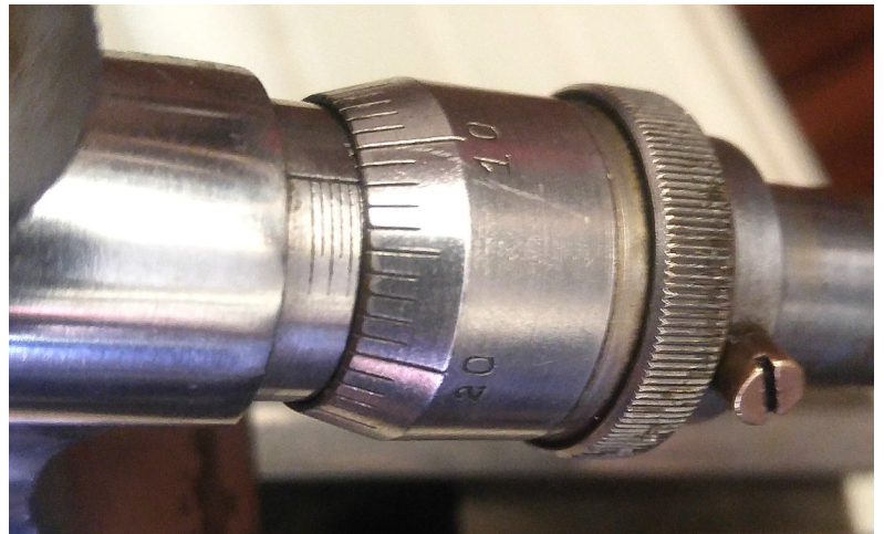
Here is a close up view of the micrometer tailstock adjustment for depth control.
