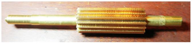
Shown here is the glued up stack with all 16 cuts completed. The tooth mesh was checked and the pinions then separated. To separate the 6 pinions I gently heated the glued stack with a propane torch to soften the superglue. Separated, the 6 new pinions looked like this.
