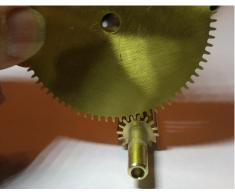
And below is a mock up of the pinions in the eventual drive train of the spring powered motor.
