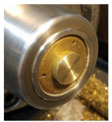
These slugs were surfaced on both sides while held in a customized brass emergency collet.
