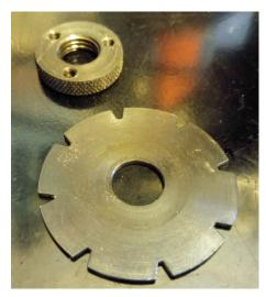
between the 8 cuts to make the final 8 cuts for a total of 16.
