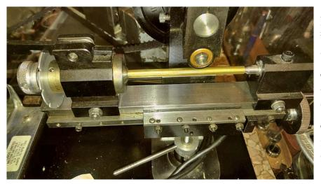
A 1/4" diameter brass rod was prepared to support the pinion blanks while they were being cut.
