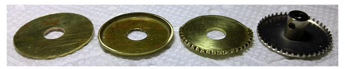
In use, this new shallow crown gear will have a very short mounting hub. All of this stubby construction is required as the completed spring powered device must be mounted into very cramped quarters. Space is at a premium.
