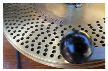
The low profile 48 pitch crown gear needs to have 44 teeth on a 1" diameter blank so I set up the wheel engine index disc for the 88 hole pattern and would use every other hole.
