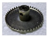
This is an "upgrade" slot car crown gear from a few decades ago. It is impossible to run a manufacturing business relying on no longer made parts to use in my products – so I had to make my own crown gears.
