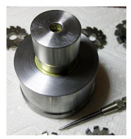
The plunger is slid over the guide rod and onto the brass washer.
