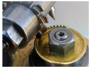
Since the custom crown gear that I require for my product will provide intermittent movement, I require only half of the crown gear to have teeth. The other half of the crown rim is ground off to provide a pause in the motion of the device. The stages of the crown gear production are shown below along with the slot car gear.
