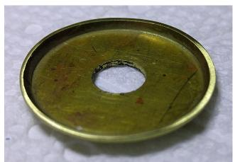
This turned up rim will have the small gear teeth cut into it to resemble the slot car gear.
