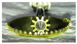
The missing tooth section of the crown gear is clearly visible in these pictures. This crown gear drives the pinion.
