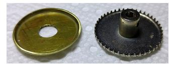
The teeth are cut using my Chronus clock wheel engine – one tiny tooth at a time. The small machinist's clamp is used to limit the depth of cut when cutting the gear teeth.
