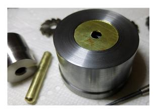
The brass guide rod is placed down through the washer and into the base.
